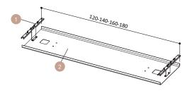
Fixing brackets with high capacity cable tray for bench desks with 38mm middle gap
