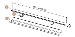
Fixing brackets with full length flap and cable tray for single desks
