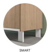
Rectangular 20x60mm 150mm high metal leg supplied with 0-15mm adjustable ø25mm levellers. Profile and cladding side panels are required.
