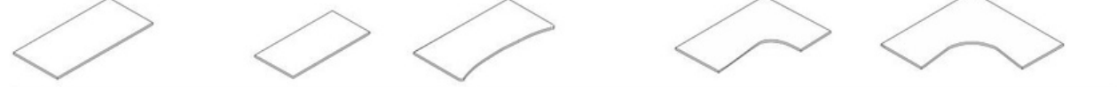
Scrivanio base/ Desk basic L 80/100/120/140/160/180 P 80 Dattilo/ Typing desk L 80/100/120 P 60 Scrivanio ergonomica/ Ergonomic desk L 90/120/140/160/180 P 90 Scrivanio corner/ Corner desk L 120 Scrivanio corner/ Corner desk L 160/180
