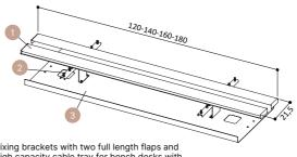
Fixing brackets with two full length flaps and high capacity cable tray for bench desks with 215mm middle gap
