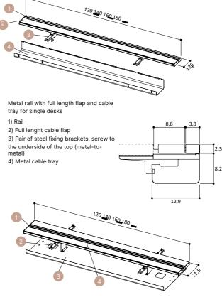
Metal rail with two full length flaps and high capacity cable tray for bench desks with 215mm middle gap
